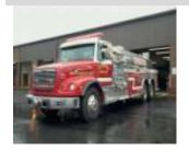
Year of Manufacture 2002 12,503 Mileage Hours 194 Can Function as Engine Tanker use only Pumping Capacity 1,500 gpm Tank Capacity 3,200 gallons Seating Capacity 3 Number of SCBA 2 Equipment Portable dump tank Surface Rust None Structural Rust and Corrosion None Apparent Fluid Leaks None Appearance and Condition Good
